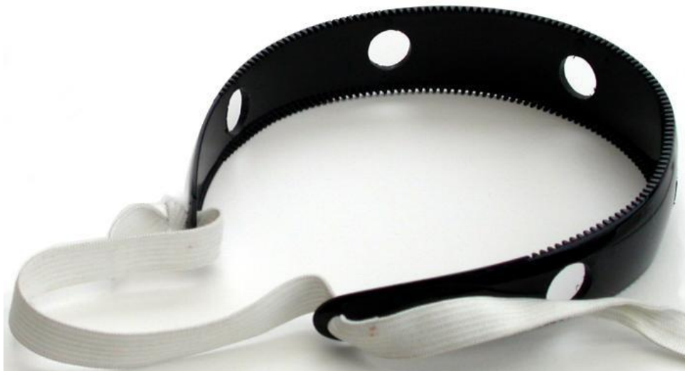
Figure 3-7: DIY Electrode Headband; An image showing the headband used for an EEG sensor mounting; reprinted with permission from OpenEEG
