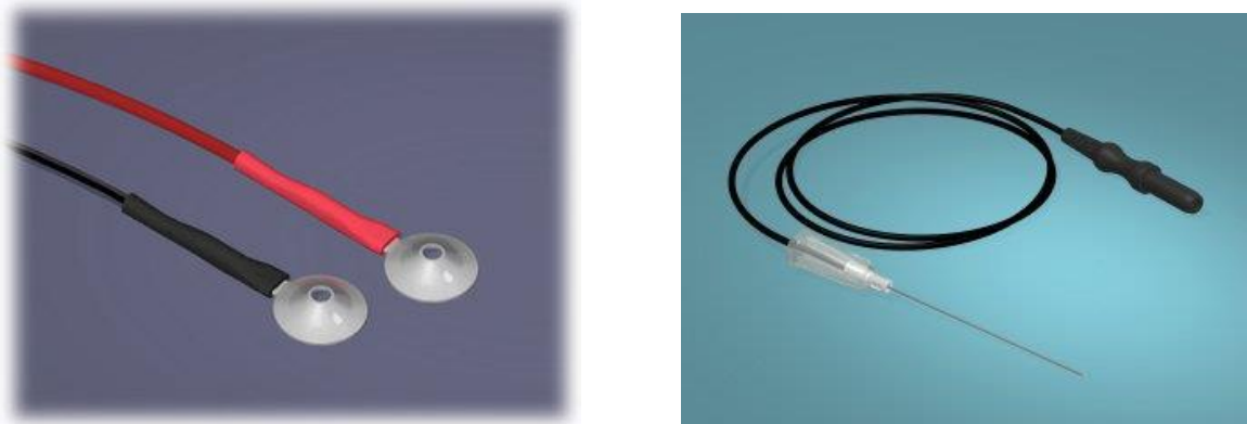
Figure 3-9: Electrode Classifications; An image demonstrating the physical differences between surface electrodes and needle electrodes; reprinted with permission from Richard Kaiser
