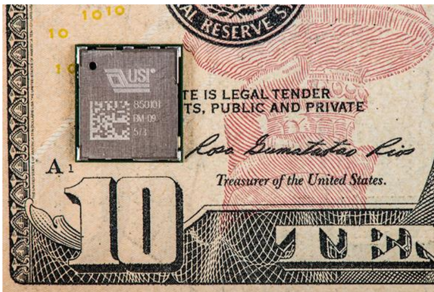
Figure 3-21: The Photon Size Reference; An image demonstrating the relative size of The Photon Wi-Fi module; reprinted with permission from Kevin @ Spark
