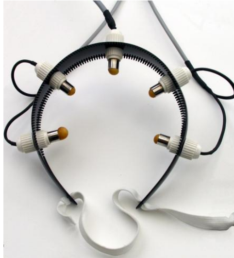
Figure 3-8: Final DIY Electrode Sensor Array; An image showing the final version of the DIY sensor array; reprinted with permission from OpenEEG
